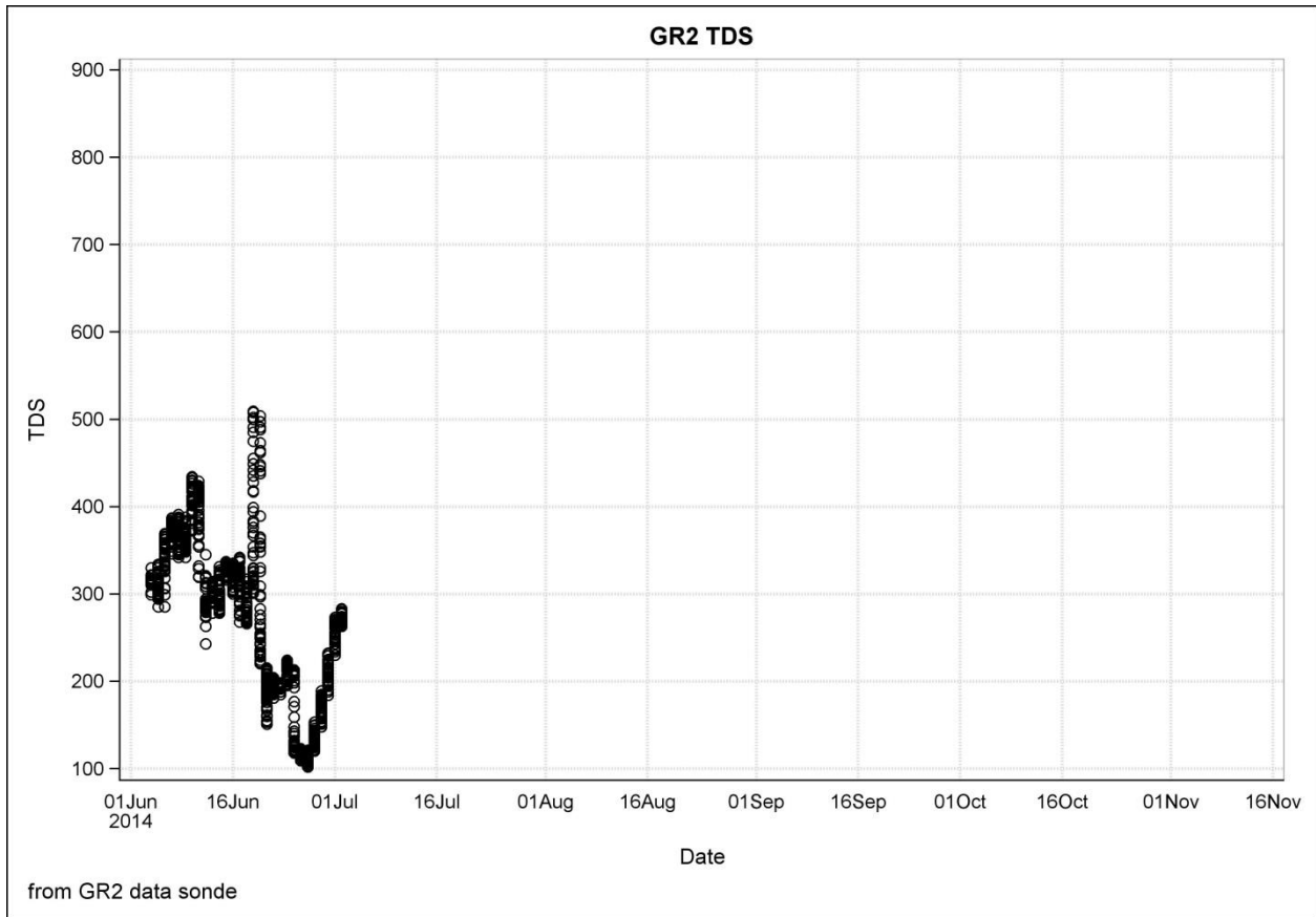
Figure A2-36. Grand River Total Dissolved Solids (TDS) 2014 data from data sonde at station GR2. Sonde probe failed on July 2 and failure was not discovered until August. No replacement was made at that time.
