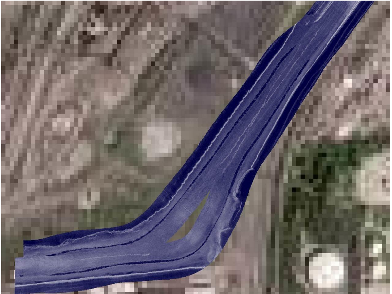
Figure 33f. Side scan habitat sampling of Cuyahoga River ship channel using Humminbird side-scan sonar and Dr. Depth mapping software: head of Navigation Channel at Arcelor-Mittal (going downstream as you go right and up in the figure; north up). The dark blue lines in the river channel represent the (two) center track paths of the boat measuring the water column as it collected side scan data.
