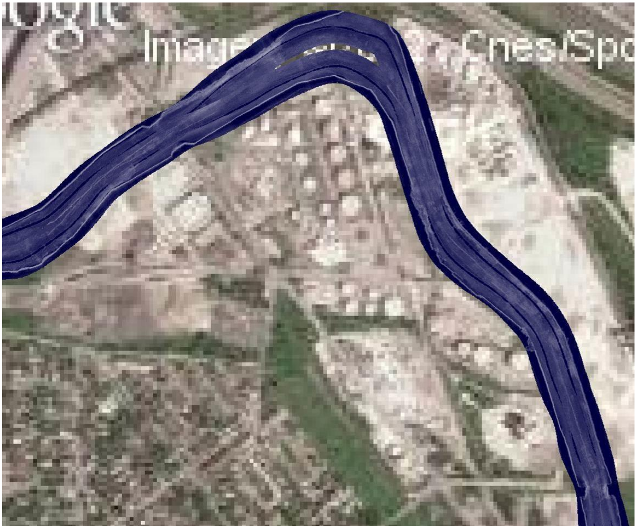
Figure 33i. Side scan habitat sampling of Cuyahoga River ship channel using Humminbird side-scan sonar and Dr. Depth mapping software: the area upstream of I-90 at Marathon Bend and the W 3 rd Street bridge (upper left). Mapping reveals uniform bottom depths and deep-water armored shores with the exception of a few bridge abutments (notched areas, bottom right and upper left) and a shallower, diverse rocky area after Marathon Bend but before the 3 rd St bridge on the right descending bank above (near the word “image”).
