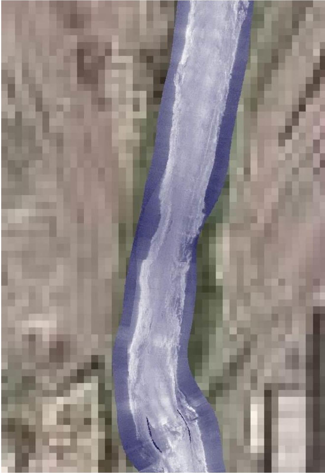
Figure 33m. Side scan habitat sampling of Cuyahoga River above the ship channel using Humminbird side-scan sonar and Dr. Depth mapping software: the concrete channel area upstream of the previous figure showing more habitat complexity.
