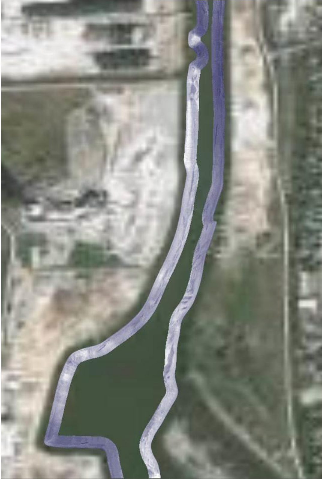
Figure 33o. Side scan habitat sampling of Grand River above the ship channel using Humminbird side-scan sonar and Dr. Depth mapping software: from the head of the Navigational channel (below) downstream to salt dome loading area (above) showing habitat areas along the margins of the ship channel.
