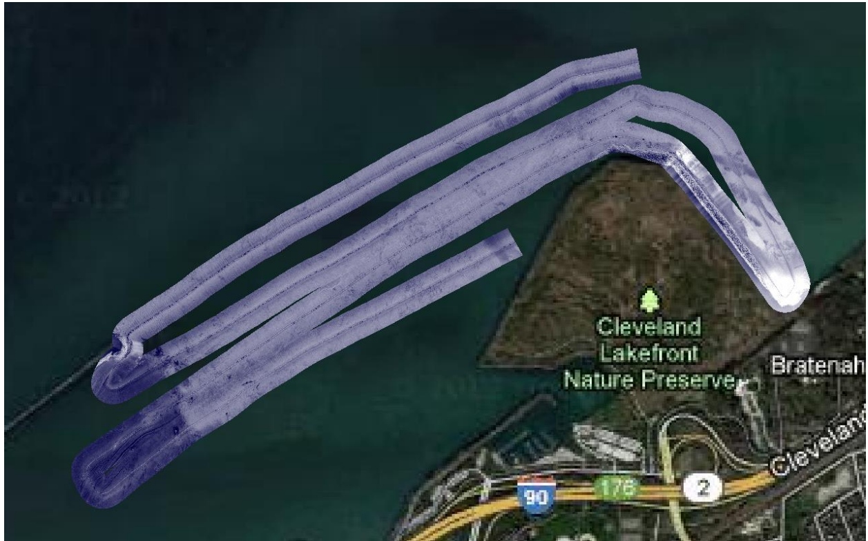
Figure 33a. Habitat mapping swath of eastern portion of Cleveland Harbor using Dr.Depth software program from data acquired from Humminbird side scan sonar. Brighter areas are shallower with more coarse-grained materials, dark areas are softer sediments.
