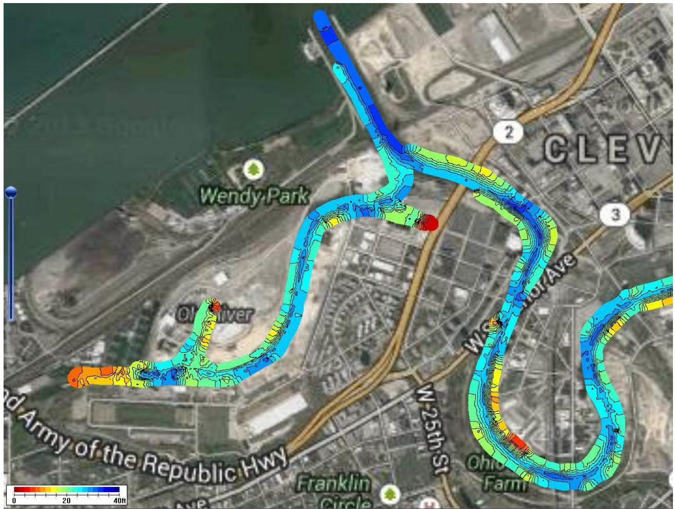
Figure 30d. Depth contour map showing depth differences between the area around Columbus Rd. (at map lower right) to the river mouth and the Old Channel (at map left) on the Cuyahoga River.
