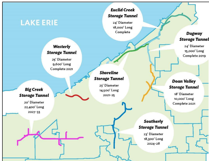
Figure 12. NEORSD storage tunnels
